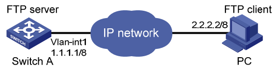
Figure 1-4 Network diagram for FTP configurations: a switch operating as an FTP server
