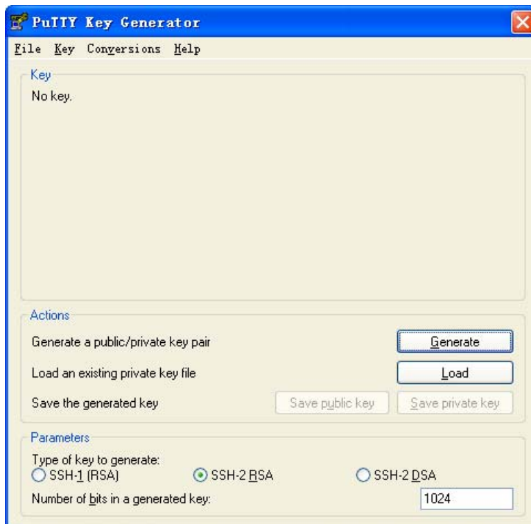
Figure 1-3 Generate a client key (1)
