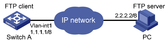
Figure 1-6 Network diagram for FTP configurations: a switch operating as an FTP client
