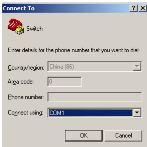
Figure 1-4 Specify the serial port used to establish the connection
